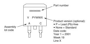
Example: This is a xxxxxxxx with assembly lot code AC, assembled on WW 19, 2001 in the assembly line "X"
