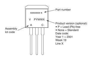
Example: This is a xxxxxxx-x with assembly lot code AC, assembled on WW 19, 2001 in the assembly line "X"
